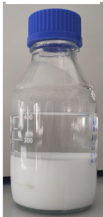
Figure 6: Product bottom up, fast synthesis method. 300mM Struvite, 100mM citrate.
