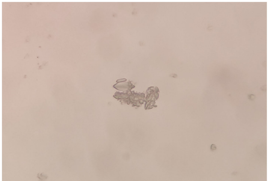
Figure 5: Microscope foto of Aggregated Struvite crystal, created by spray synthesis. Picture taken through a 400x microscope lens.
